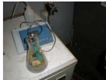
Plate 1: Testing of the medium using pH meter
